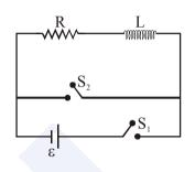
the switch  $S_1$  is closed at time t = 0 and the switch  $S_2$  is kept open. At some later time  $(t_0)$ , the switch  $S_1$  is opened and  $S_2$  is closed. The behavious of the current I as a function of time 't' is given by :
